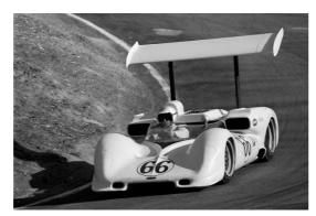
Although our previous cars took advantage of aerodynamic design for systems such as the cooling ducts, SFR10 first used aerodynamics to improve the vehicles on-track grip. The package was comprised of front, side and rear wings, with a computational fluid dynamics (CFD) estimated lift and drag coefficient of -4.0 and 1.5 relatively
